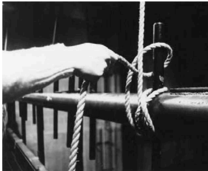
Fig. 3.33. Tying off, step 5
