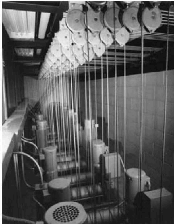
Fig. 5.1. Electric motorized winches. Courtesy of Peter Albrecht Corp.
