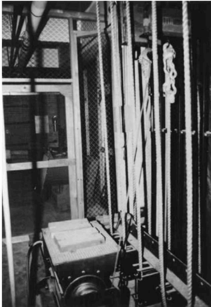
Fig. 4.42. Bull winch used to load arbor in a facility with no loading bridge
