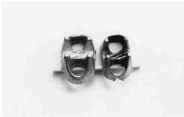
Fig. 6.15. Two malleable saddles—note differences in size and quality
