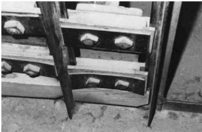
Fig. 4.19. Bent tension- block guide
