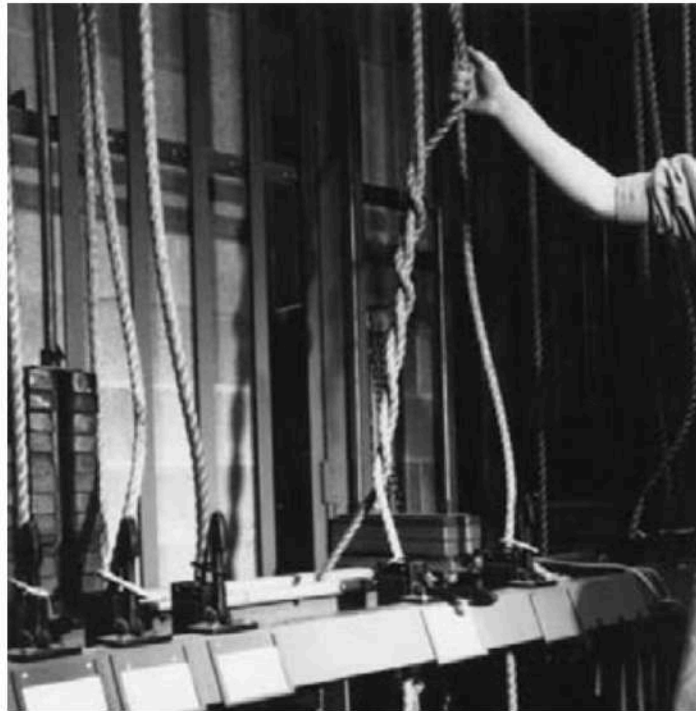
Fig. 4.31. Safety twist in hand line
