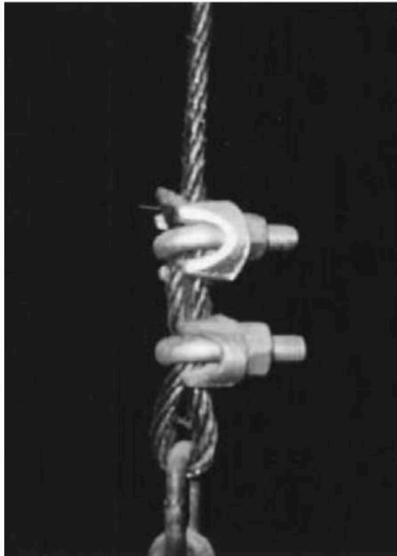
Fig. 6.16. Clips installed too close together
