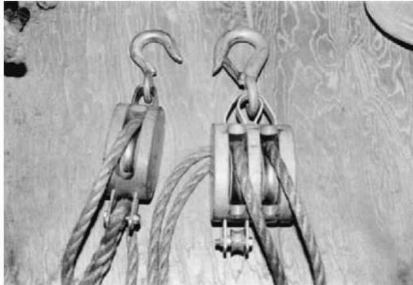
Fig. 2.14. Different-sized hooks on blocks
