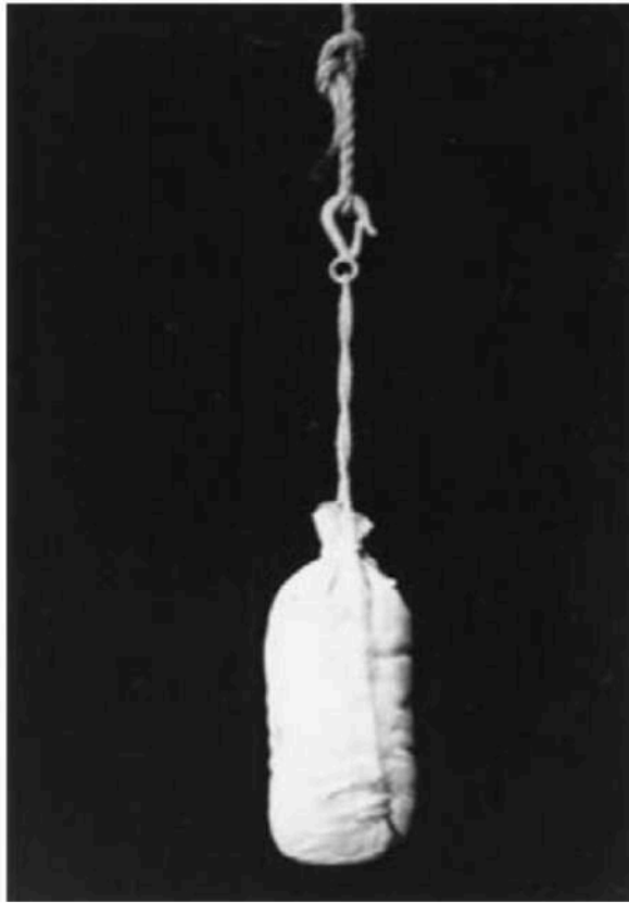
Fig. 3.46. Rope weighted with sandbag
