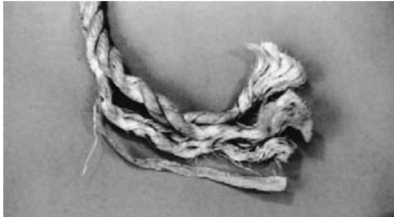
Fig. 3.7. Manila rope with identification tracer
