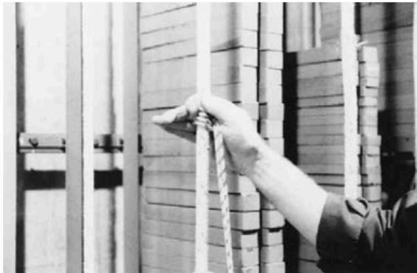
Fig. 4.35. Slipping the knot on the safety line
