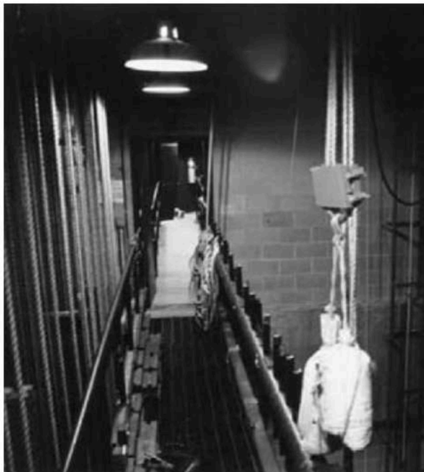
Fig. 3.6. Sandbag on a trim clamp
