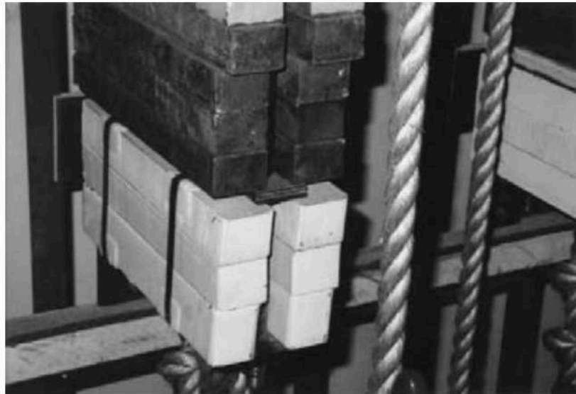
Fig. 4.23. How not to use spreader plates
