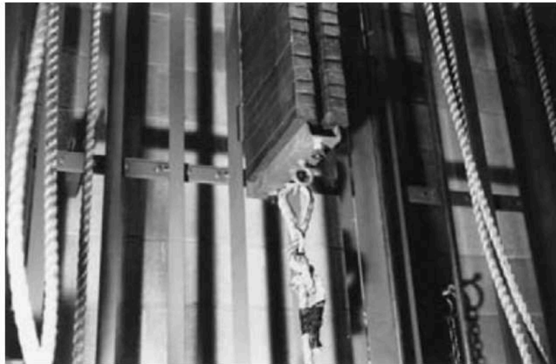
Fig. 4.26. Hand line tied at arbor bottom
