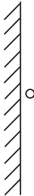
Figure 16-25. A simple spherical source located very close to an ideally infinite rigid barrier.
