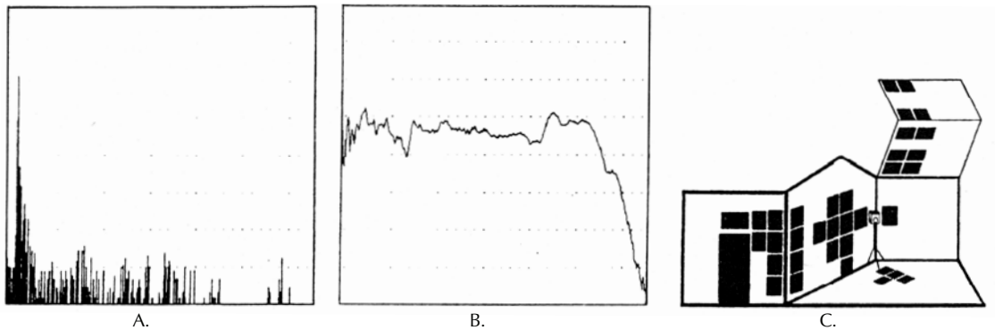
Figure 13-22. Effect of Sonex being added to the small room in Fig. 13-21. (Courtesy Doug Jones.)
