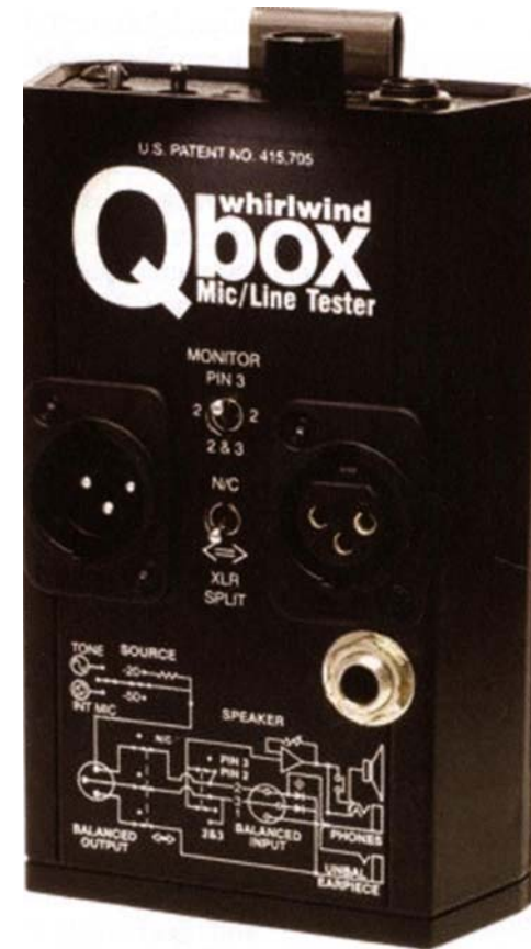
Figure 8.5 Listen box. Headphones or speaker can be plugged into the output. Any point in the signal path can then be aurally monitored (courtesy of Whirlwind USA)
