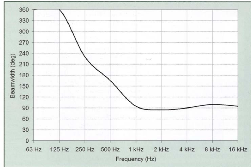
Figure 1.45 Beamwidth vs. frequency of a small-format full-range loudspeaker. Coverage angle is 90 degrees (nominal)
