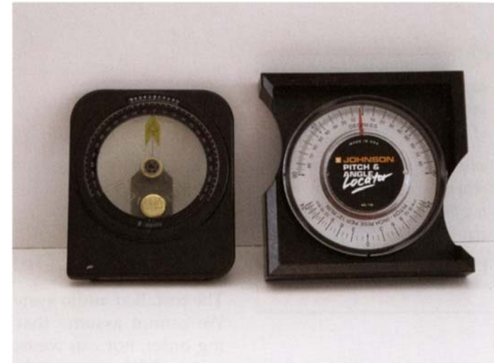
Figure 8.1 Inclinometers used for speaker vertical angle adjustment and verification
