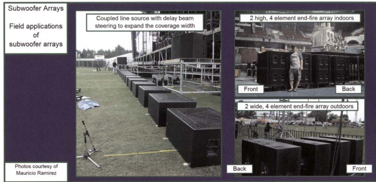
Figure 6.65 Subwoofer configuration photos
