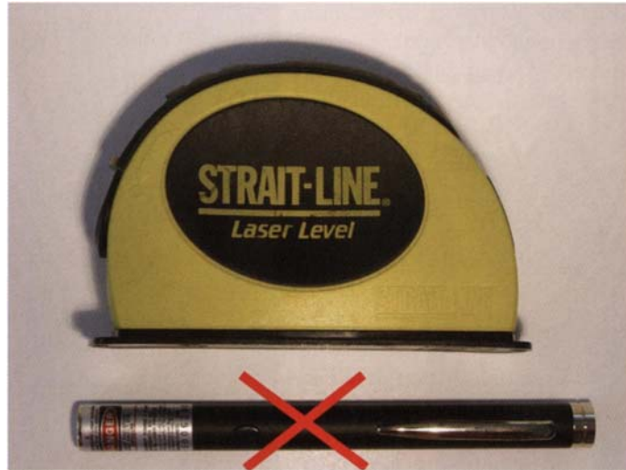
Figure 8.4 Laser pointers. The upper unit is manufactured to tolerances suitable for optimization. The presentation quality device is not suitable
