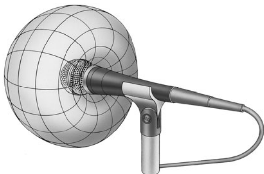
Figure 3.2 Super-cardioid pickup pattern. Image courtesy of Shure Inc.
