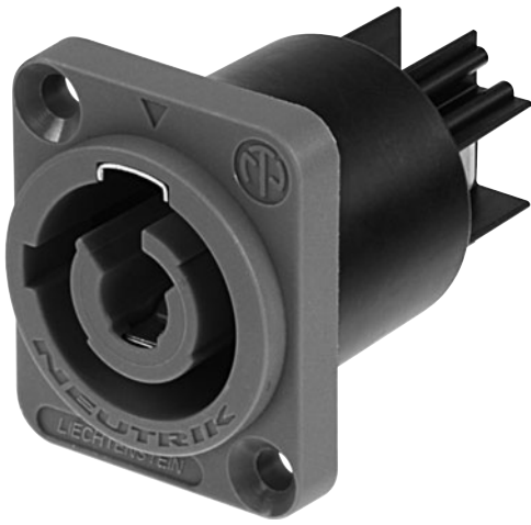
Figure 4.10 A powerCON receptacle. Note the slot. The connector can only be inserted one way, and once inserted, a twist locks it in place. Image courtesy of Neutrik.
