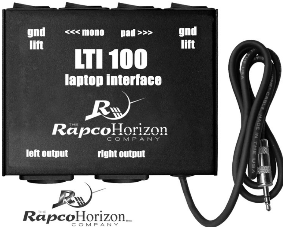
Figure 3.6 The Rapco LTI 100 is one of several purpose-built direct interfaces. This one is for getting a computer, iPod, or other device with an 1/8-inch stereo output into the PA on two balanced XLR connections. Image courtesy of RapcoHorizon.
