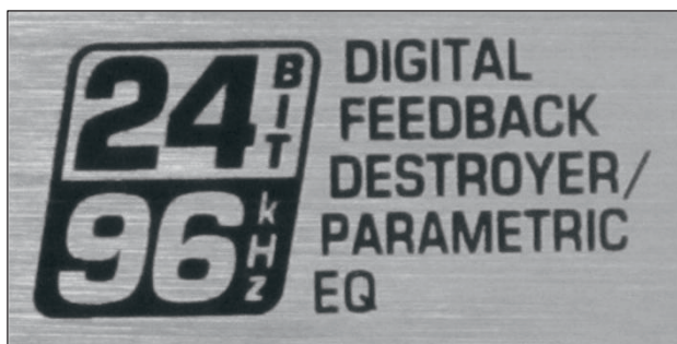
Figure 7-4 Label on Digital Processor Showing Word Size and Sample Rate
