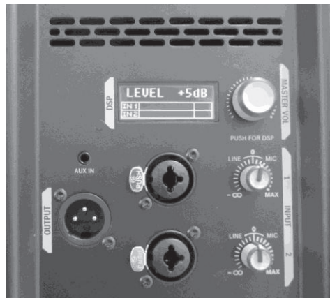
Figure 4-19 Amplifier Module Integrated into Powered Speaker System
