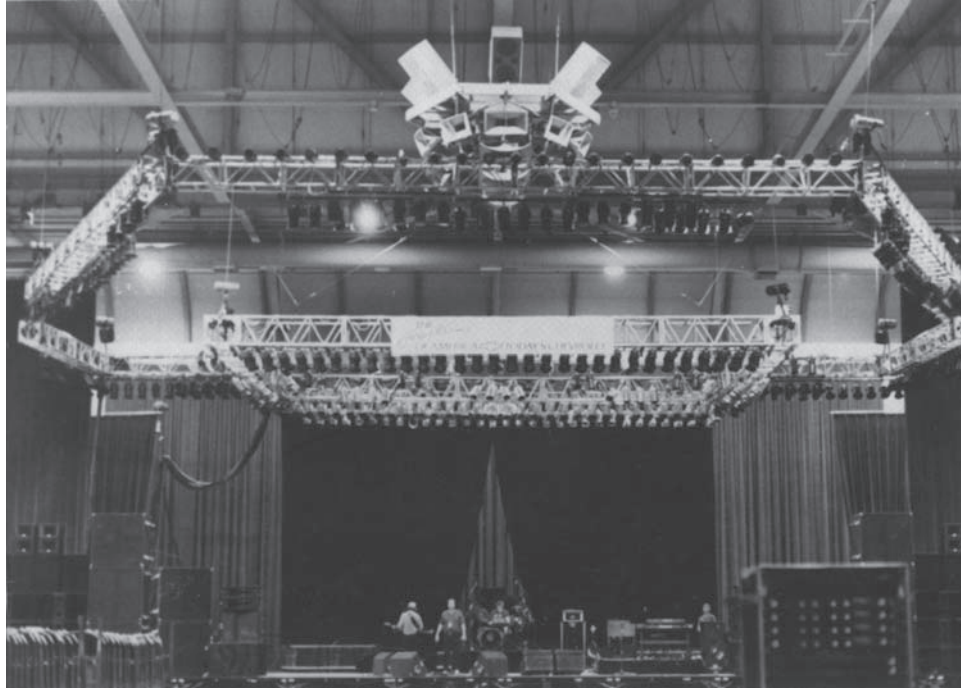
FIGURE 14.11 Truss raised with eight motors. (Photograph by Sundance Lighting Corp.)
