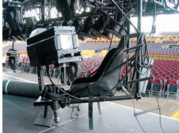
FIGURE 13.20 Spot chair setup during the 2008 Metal Masters tour. (Photograph by Paul Dexter.)
