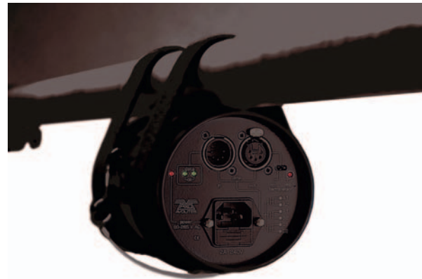
FIGURE 20.2 Truss-mounted Optosplitter. (Photograph by Avolites, Ltd.)
