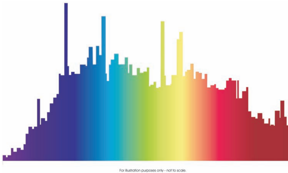
Figure 13-10 The spectral power distribution of a discharge lamp is not continuous as in an incandescent lamp. Instead, it exhibits peaks and troughs at various wavelengths.
