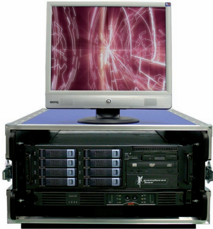
Figure 3-24 A DMX512-controlled media server stores and plays back graphic files that are fed to a display device such as a projector or LED display. Pandora's Box is one example of such a media server.
