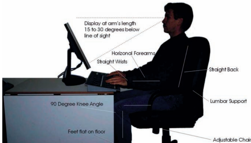
Figure 22-1 An ergonomically correct front of house (FOH) set up is very important for the long-term health of a programmer.
