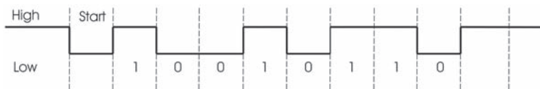
Figure 15-2 A DMX512 signal is a series of high and low voltages, which makes a square wave.
