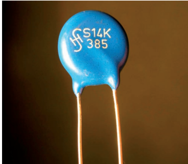
Figure 8-4 An MOV is a type of diode with certain characteristics that make it ideal for overvoltage protection.
