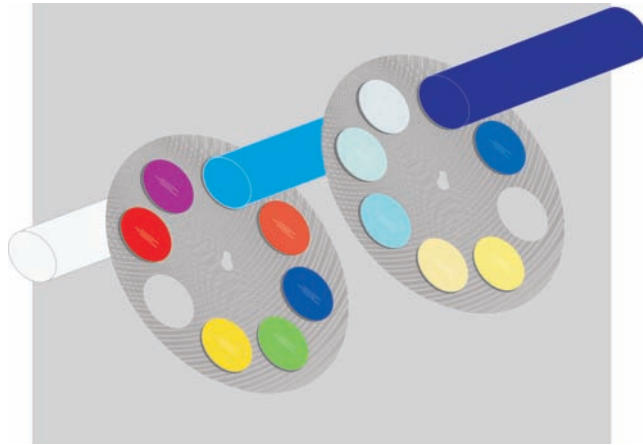
Figure 14-16 By adding a secondary color wheel with carefully chosen colors, the number of available colors in an automated fixture can be multiplied.
