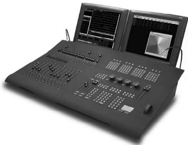
Figure 1.8 A Computer Lighting Console
